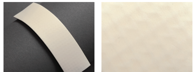
Versico VersiWeld – 60 Weeks (No Failure)
